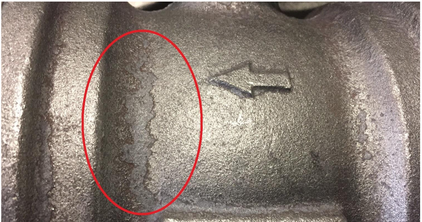
Figure 1.6.4 – Example of unacceptable casting voids
