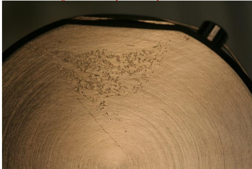
Figure 1.8.3 – Examples of Pitting
