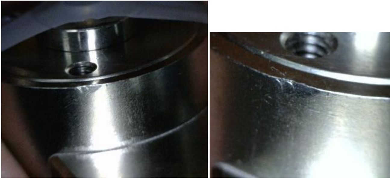
Figure 1.4 - Example of Unacceptable Chatter
