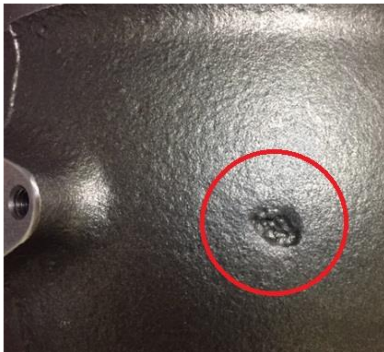
Figure 1.6.4 – Example of unacceptable casting voids
